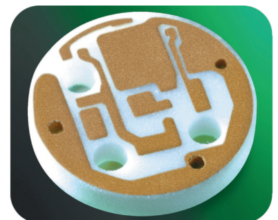
Thick-film Au with 75µm track/gap
