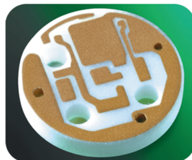
Thick-film Au with 75µm track/gap
